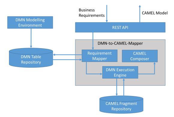
Figure 18 - DMN-to-CAMEL-Mapper high level architecture
