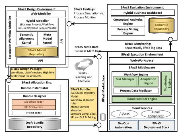
Figure 1 Context to the architecture of the CloudSocket platform
