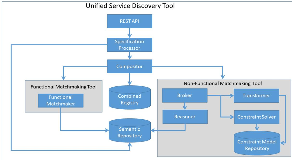
Figure 43: The architecture of the Unified Service Discovery Tool
