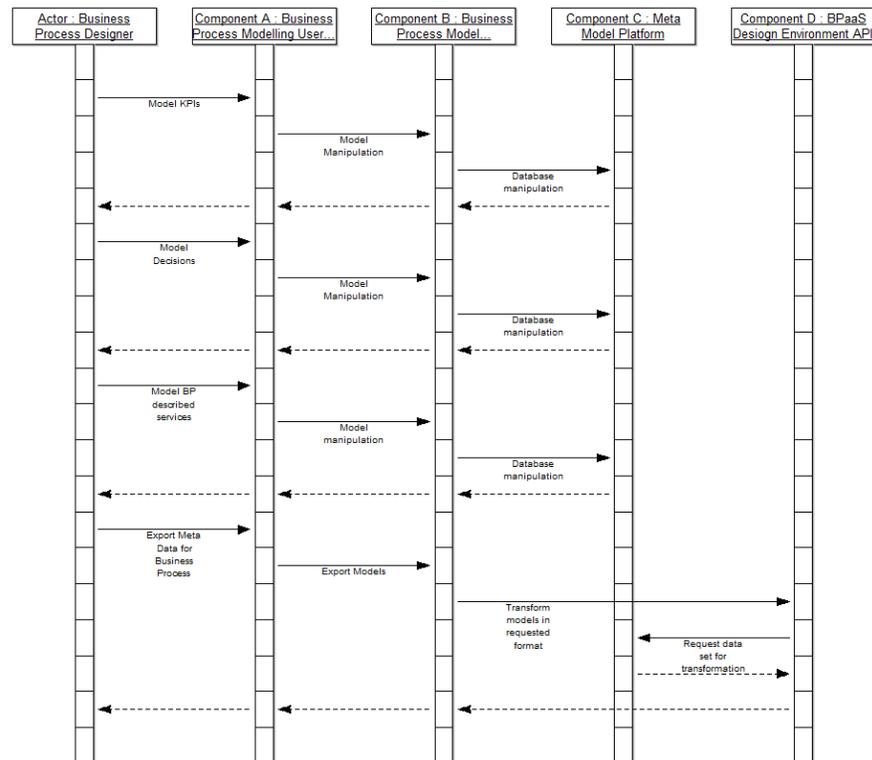
Figure 14 Sequence Diagram – DE-UC-5-KPI Definitions and Meta Model Completion
