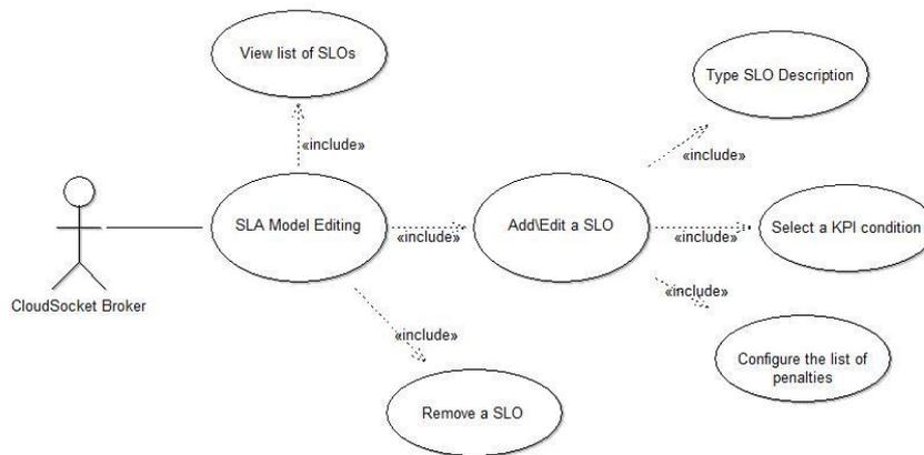
Figure 32 Use Case Diagram – AE-UC-5-SLA Model Editing
