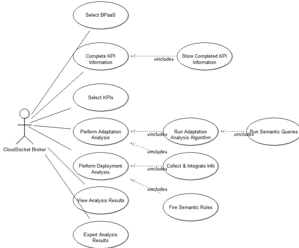
Figure 78 Use Case Diagram – EvE-UC-2-Derivation & Visualisation of Best Deployments and Adaptation Patterns/Rules
