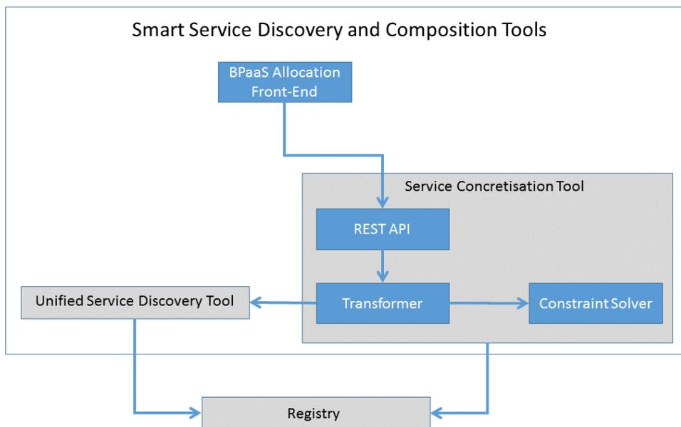
**Figure 42: The architecture of the Smart Service Discovery and Composition Tools**
