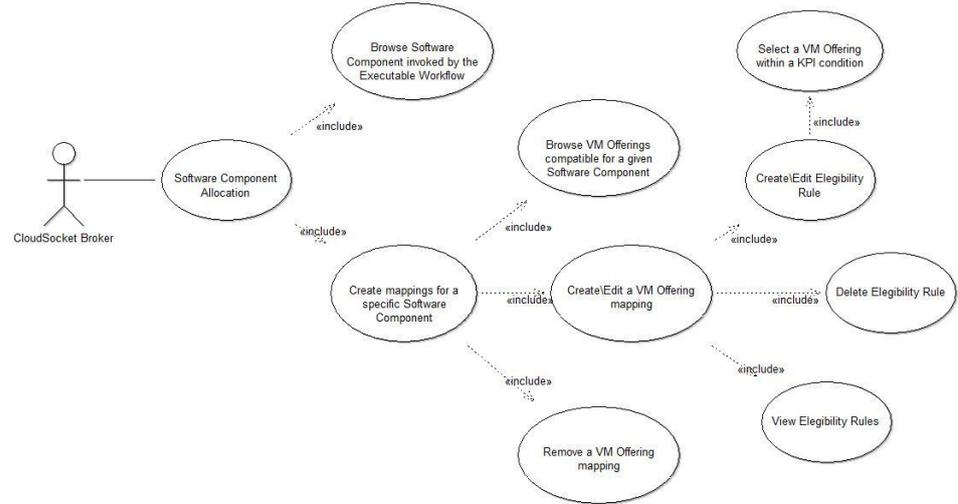
Figure 28 Use Case Diagram – AE-UC-3-Software Component Allocation
