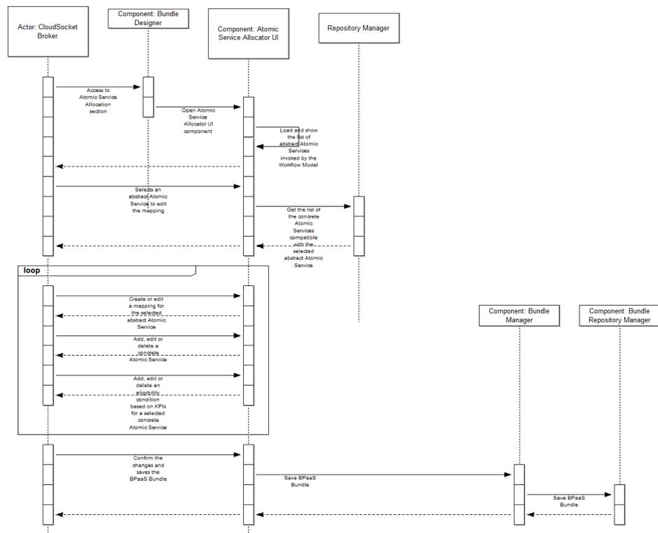
**Figure 27 Sequence Diagram – AE-UC-2-Atomic Service Allocation**
